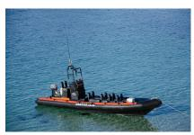
Connachar with its deep v hull makes for a comfortable ride in most sea states. The front seats are all removable to give large amounts of deck space for carring up to 1000kg in cargo. The cowains driving position is raised at the stern to give very good visibilty, with a wrap around screen to give added protection.
