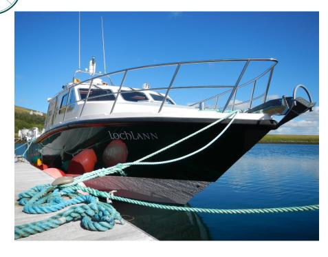
Lochlann is powered by twin Caterpillar 3126 diesel engines, supplying 426 horsepower each, which gives a top speed of 27 knots and a cruising speed of 17 – 18 knots. Its well-apportioned interior provides spacious seating for 12 people.
