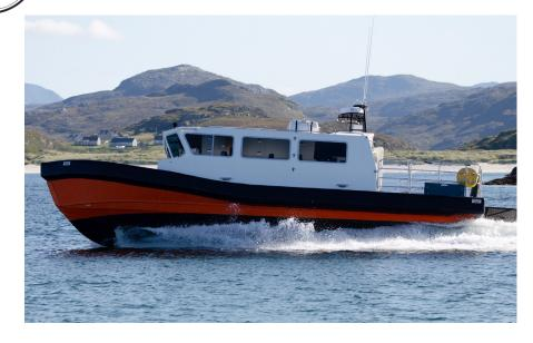
Challenger is powered by twin Yanmar 315hp diesel engines, supplying a total of 630 horsepower, which gives a top speed of 30 knots and a cruising speed of 22 knots. Its well-apportioned interior provides spacious seating for 15 people.
