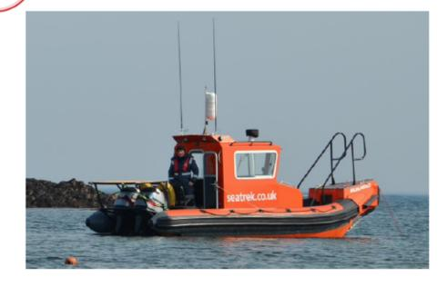
Highlander has been purpose built for Seatrek. At 7.4m long it can be towed by a 4x4 and is easily managed by two people for launching and recovery. This vessel is ideally suited for quick response situations. It has been designed around the proven Delta ribs which Seatrek have operated for many years. Within the cabin area there are 4 seats to give comfort in most conditions. Outside seating consists of removable bench seating for 4.
