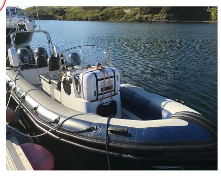
XS 7 metre RIB Yamaha 80 hp x 2 Comfortable seating up to 10 Long range fuel tanks MCA (CAT 3) 20 miles 8 +2 persons G.P.S. (for accurate location) Chart Plotter (for accurate navigation) V.H.F. Radio communication x 2 D.S.C. (Emergency location positioning) Life Raft for 10 persons Talisker comes with its own road trailer
